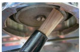
95.01773 ) supplied with the machine, to eliminate coffee residues from the filters and showers
